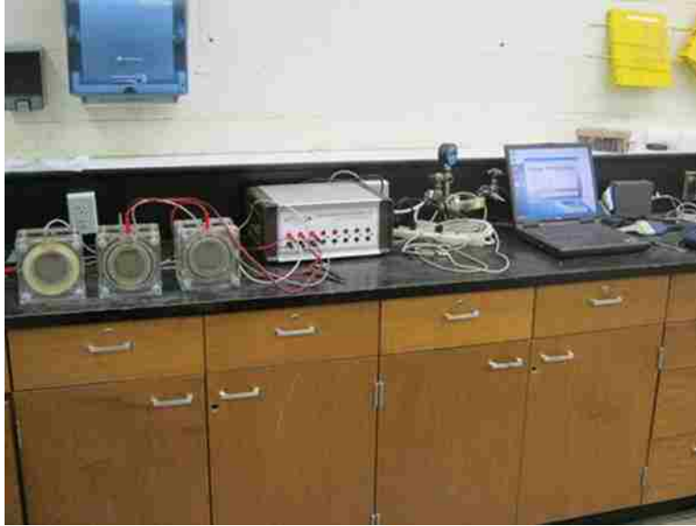
Figure 3-16: Rapid chloride permeability testing apparatus.
