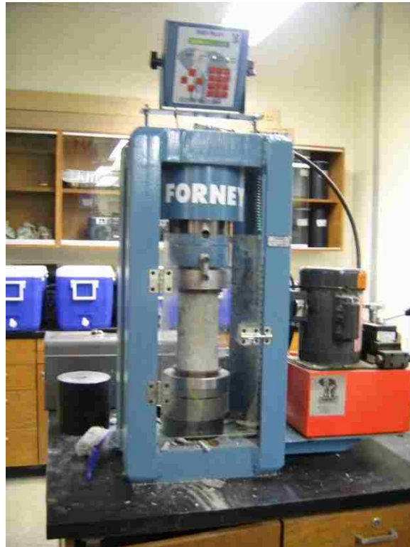
Figure 3-15: Compressive strength testing.
