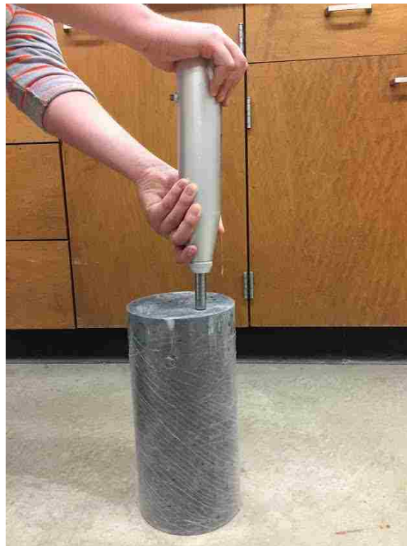
Figure 3-18: Schmidt rebound hammer testing.
