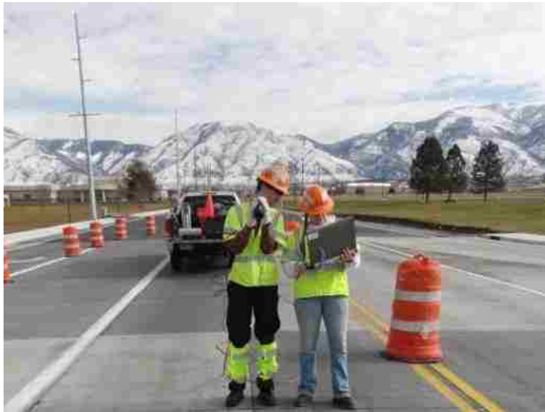
Figure 3-10: Measurement of surface temperatures using infrared thermography.
